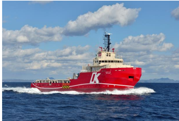
[Work Vessel for Offshore construction (AHTSV*3 Offshore Operation Co, "Akatsuki")]
