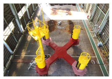
A scale model, which was fabricated based on the JMU original design, will be installed off the coast of Akita-city and Katagami-city, and moored by hybrid mooring systems, which are formed by combinations of steel chain and fiber rope. Robustness assessment for mooring systems, methodology for designing mooring systems and its constructability will be validated. Please refer to the "Outline of demonstration project" below for the details.
